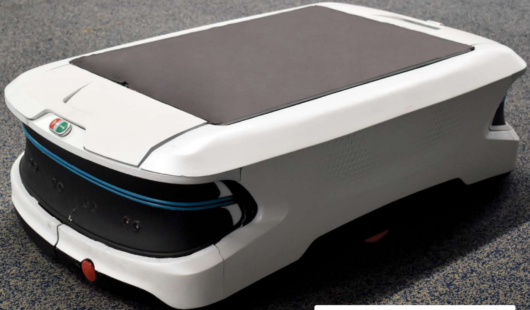
Cynor, the smart robotic warehouse keeper of Digikala which is used for transferring various goods, pallets, shelves and handwheels in fulfillment centers.
